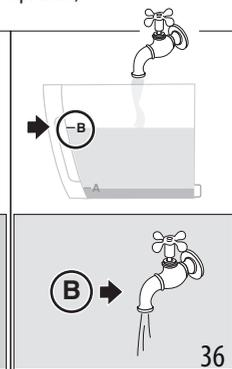
4. Pour the descaler «C2» into the tank up to level **A** (corresponding to a 100ml pack) marked on the inner surface of the tank «fig. 35», then add a litre of water up to level **B** «fig. 36» and put the water tank back in the appliance.
