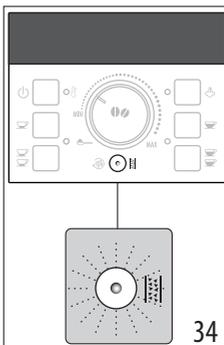
Descal the appliance when the
